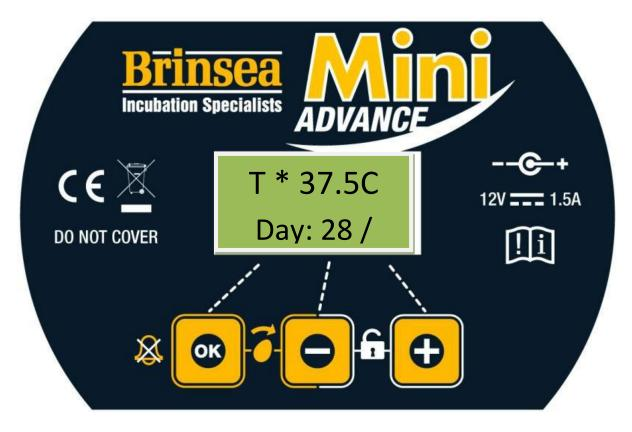
Normal operation – Temperature, number of days remaining until the hatch is due and turn system status are continuously displayed.
